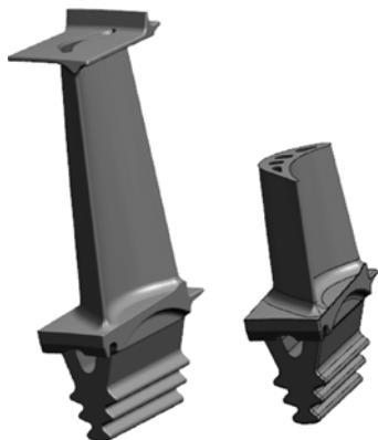
图 8 原涡轮叶片与截短后的涡轮叶片对比 Fig. 8 Comparison of original turbine blade and cutted turbine blade
